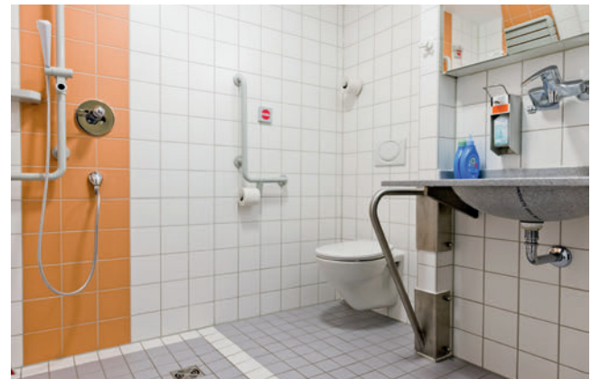
Fig 2.5-9 Patient bathroom free of obstacles, equipped with plenty of handlebars and enough room for the patient, a nurse, and an occupational therapist, along with auxiliary material.
