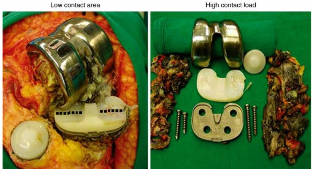
**FIG. 5.105** *Left*, Intraoperative photograph of TKA with catastrophic wear after 9 years. Flat PE bearing articulating with a flat-style femoral component. This allows for only a thin line of contact (*dotted line*) during knee load. The stresses generated upon the PE are excessive, and the PE fails macroscopically. *Right*, Inflammatory debris removed at the time of revision.
