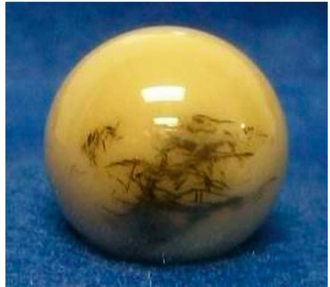
**FIG. 5.39** Photograph of a retrieved ceramic head demonstrating metal smear. With repetitive hip subluxation, metal from the acetabular cup is transferred to the ceramic head. The greater the smear area, the higher the rate of PE wear.
