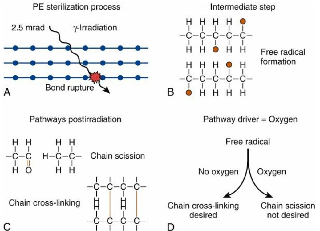
**FIG. 5.25** Diagram depicting PE irradiation process. Irradiation of PE causes bond rupture (A), which creates free radicals (B). Free radicals can combine with oxygen to create an oxidized form of PE, which results in chain scission; in the absence of oxygen, the PE chains can form cross-links (C). The presence or absence of oxygen determines the pathway the PE free radicals will take (D). Cross-linking is the desired pathway.
