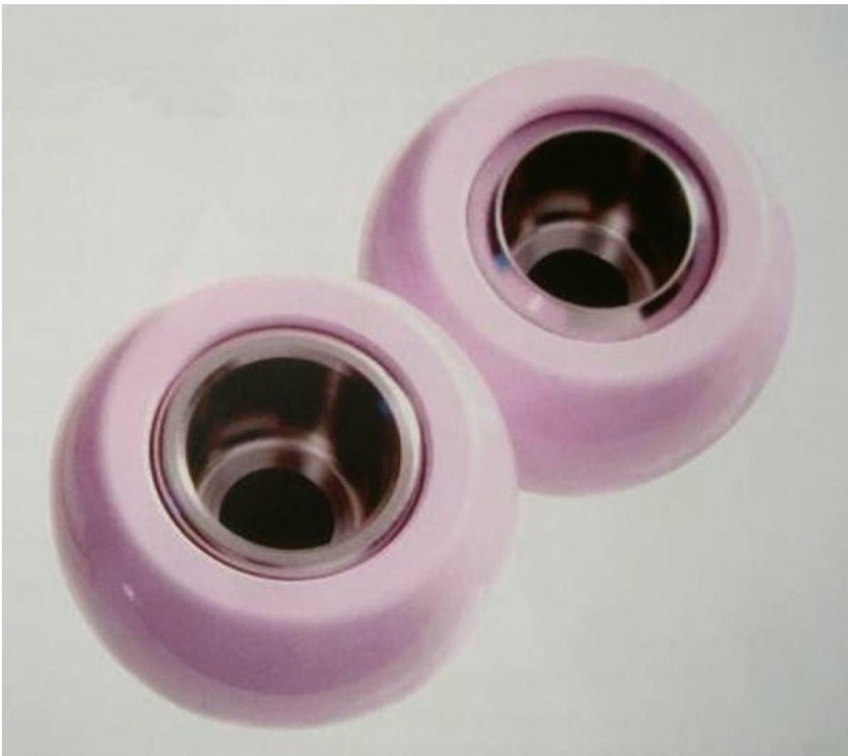
**FIG. 5.44** Photograph of internal metal jacket in ceramic head. This internal metal sleeve protects the head from burst fracture when placed on to a used femoral neck that has been roughened by use.
