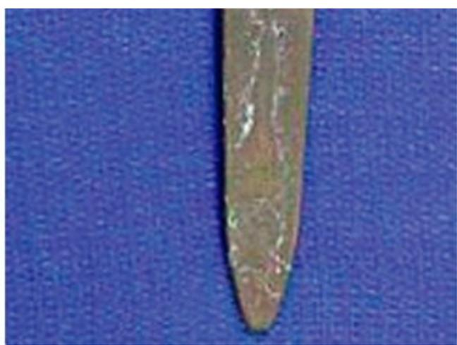
**FIG. 5.14** Retrieval photograph of bone ongrowth stem. The stem has a sharp angle wedge design in two planes. The edges of the implant are sharp to provide rotational stability. Note the rather scant amount of bone on the surface of this prosthesis. Implant was found biologically stable at the time of removal.
