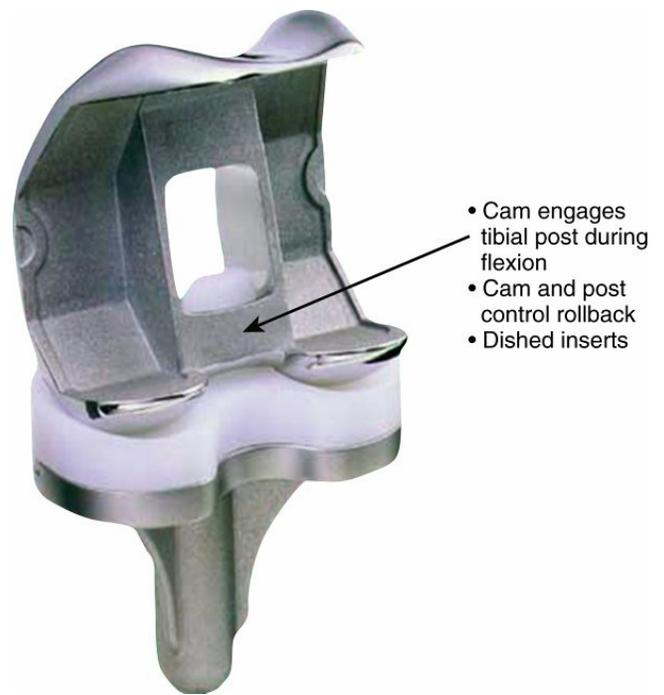
**FIG. 5.81** Posterolateral view of posterior stabilized (PS) implant. This is the typical profile of the femoral and tibial components. The cam on the femur engages a tibial post when the knee moves into flexion. This prevents anterior translation of the femur on the tibia, stabilizing the knee in flexion in the absence of a posterior cruciate ligament.
