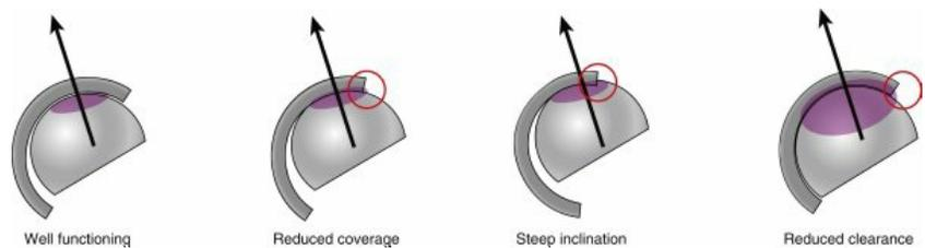
**FIG. 5.40** Edge wear occurs when the maximum area of wear crosses over the edge of the cup and has been associated with increased wear rates in metal-on-metal bearings. Potential causes of edge wear (*circles*) are shown; they include reduced coverage of the head from a cup that is less than a hemisphere, a cup that is excessively vertical, and reduced clearance between the head and the cup.
