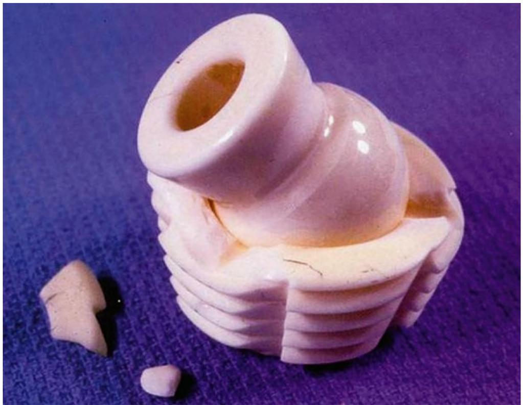
**FIG. 5.42** Photograph of retrieved first-generation ceramic-on-ceramic THA. Note very thick neck, which was required for strength in first-generation systems. The enlarged neck adversely reduced head/neck ratio. Also note acetabular fracture resulting from neck impingement.
