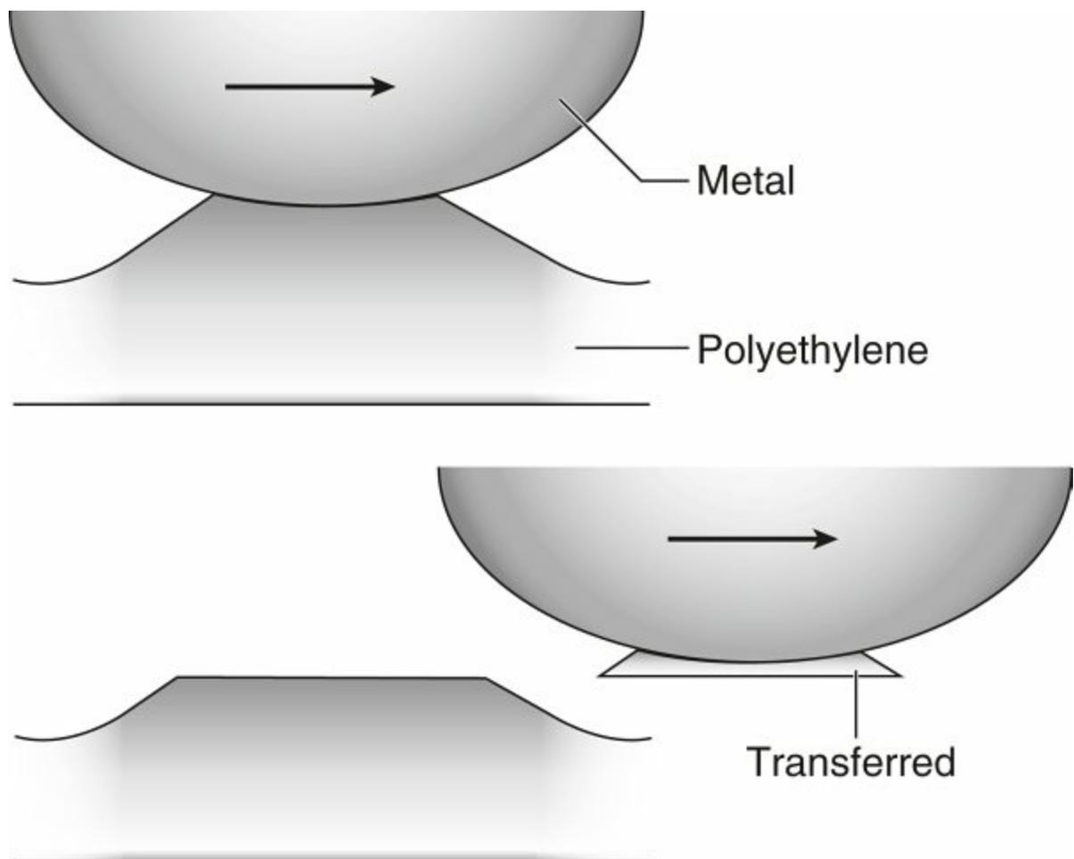
**FIG. 5.29** Adhesive wear occurs when the atomic forces occurring between the two opposing surfaces are stronger than the inherent strength of either material. In THA, adhesive wear causes small portions of the PE surface to adhere and transfer to the opposing metal femoral head. This process leads to wear particle generation and the creation of pits and voids in the PE.
