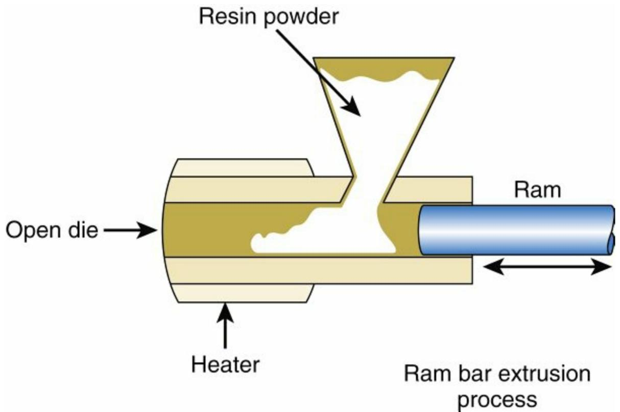
**FIG. 5.27** Diagram of ram bar extrusion process. PE powder is poured into the chamber. The chamber is heated, and the bar of melted PE is pushed out the end of the die. Calcium stearate is added to the PE powder to prevent it from sticking to the surfaces of the die.
