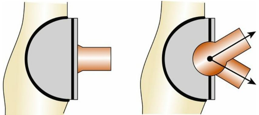
**FIG. 5.51** Diagram of constrained acetabular cup. A constrained liner covers the femoral head past its equator. This keeps the ball from coming out of socket but has the adverse effect of severely restricting primary arc range.
