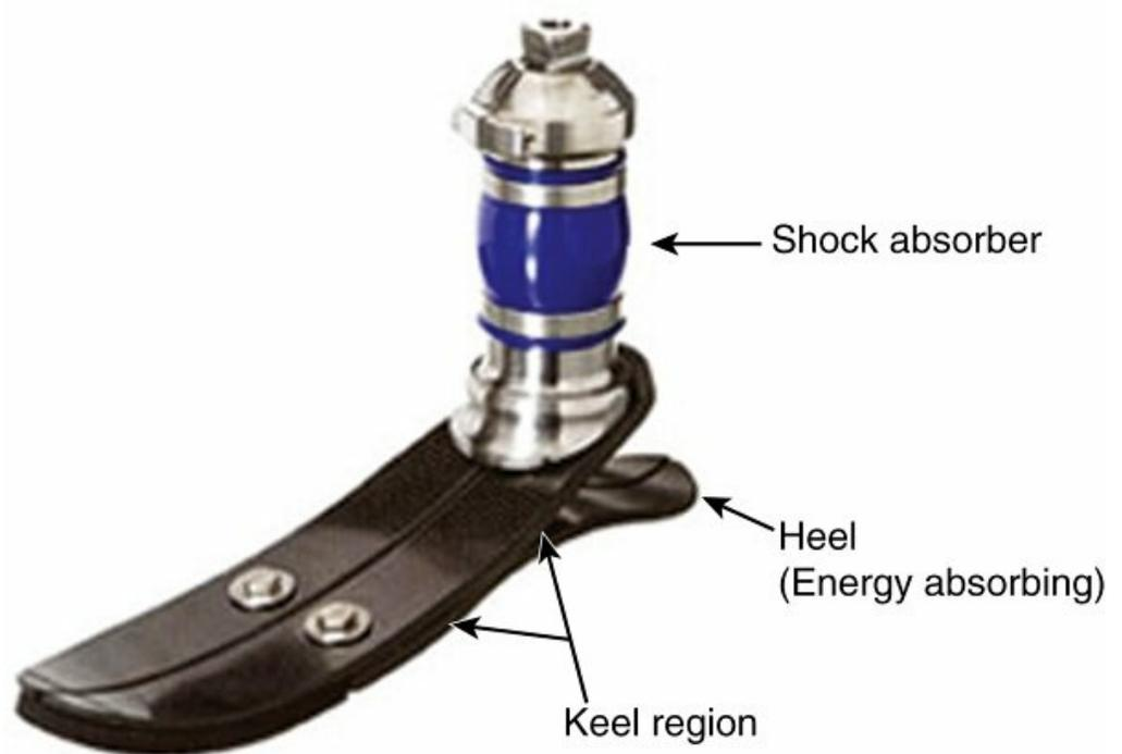
**FIG. 10.10** Ceterus prosthetic foot with leaf spring and shock absorber.
