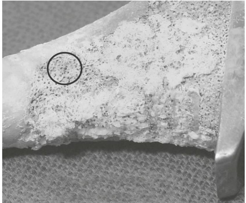
**FIG. 5.11** Ex vivo retrieval of bone ingrowth femoral stem. Note metallic pores (*circle*) that allow bone to grow into prosthesis and osteointegrate.
