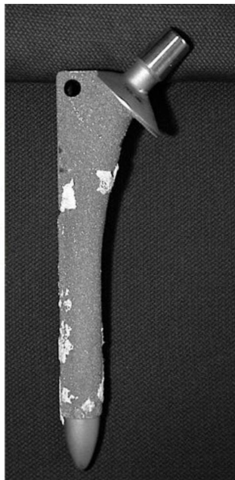
**FIG. 5.16** Diagram and retrieval photograph of distal bone loading in an extensively porous-coated prosthesis. With extensive porous coating, a majority of bone ingrowth occurs in the femoral diaphysis. Loading forces are transferred through the porous coating into the more distal diaphysis. As a result, bone density in the proximal femur is reduced because it does not experience as much load.
