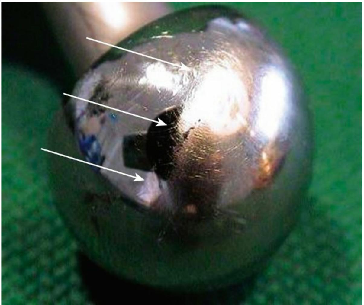
**FIG. 5.36** A retrieved cemented femoral stem with nonmodular titanium femoral head. *Arrows* point to hemisphere of abrasive wear. This area articulates with the PE cup. It has become scratched by third-body particles that have entered the joint-bearing region. This roughened surface greatly increases PE wear.
