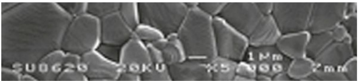
**FIG. 5.38** Scanning micrograph of surface of a ceramic head. Note residual pits (*circle*) on surface. These small areas create the roughness of a ceramic surface.
