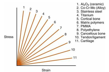
**FIG. 1.61** Comparison of Young's modulus (relative values, not to scale) for various orthopaedic materials.  $\text{Al}_2\text{O}_3$ , Alumina; Co-Cr-Mo, cobalt-chromium-molybdenum; PMMA, polymethylmethacrylate.
