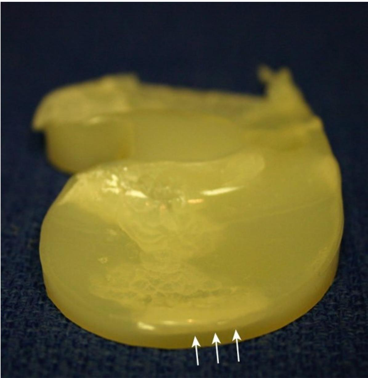
**FIG. 5.109** Retrieved PE knee insert after 9 years in vivo. Note classic white band of oxidation located 1–2 mm below machined surface of PE (*arrows*). The knee was revised for catastrophic wear.
