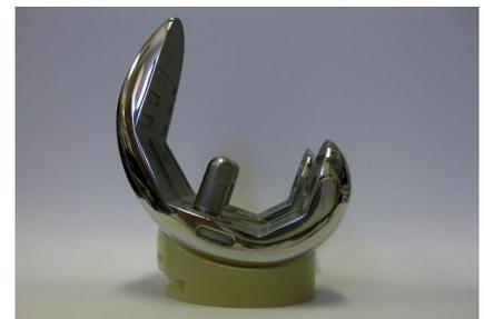
**FIG. 5.86** Lateral view of anterior stabilized (AS) TKA design. This is the typical profile of the femoral and tibial components. The tibial PE bearing is highly congruent and also has a raised anterior PE lip and a smaller posterior lip to resist anterior translation. In this design there is minimal rollback.
