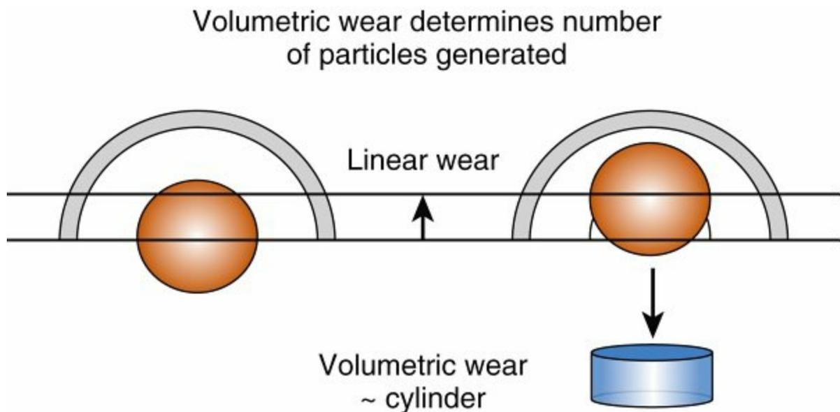
**FIG. 5.33** Diagram of PE wear in THA. As the head wears through the PE cup, a wear track is generated. Liner wear is measured where the femoral head has penetrated into the PE cup. The wear track generated approximates a cylinder.
