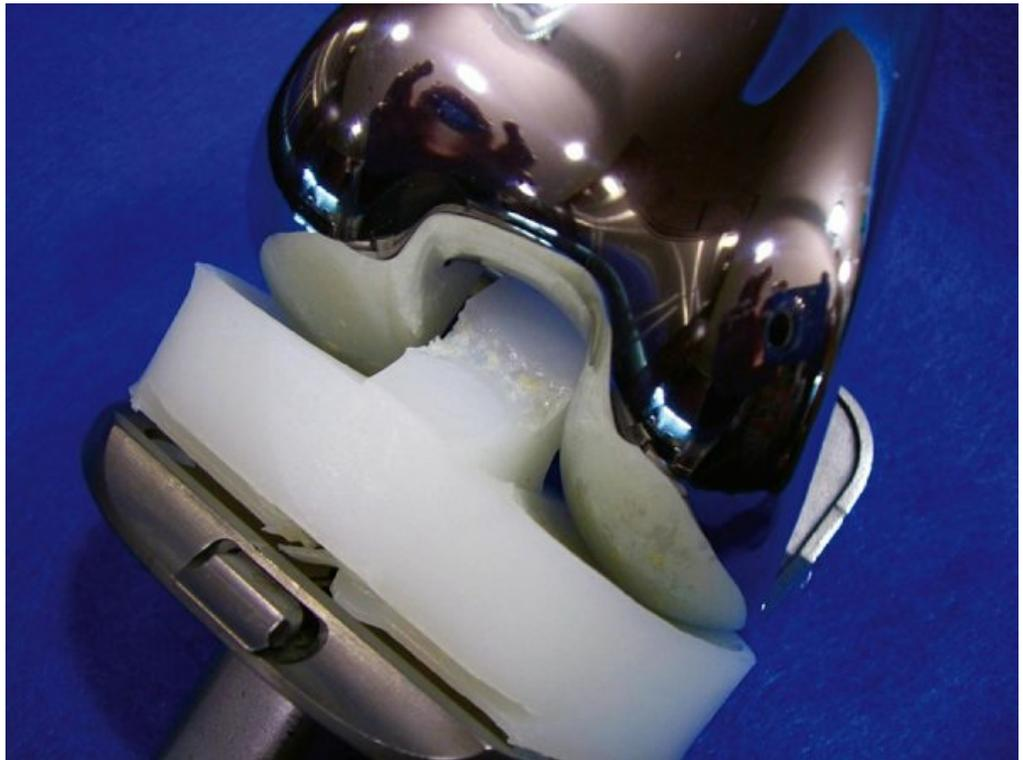
**FIG. 5.85** Photograph of posterior stabilized implant with anterior tibial post wear. Note indentation on anterior post where the edge of femoral box impinges upon it. This occurs when the knee moves into hyperextension.
