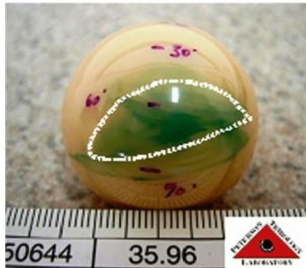
**FIG. 5.43** *Left*, Diagram depicting stripe line. With repetitive subclinical subluxation, the prosthetic head rotates upon the edge of cup bearing. This is a high-contact-stress scenario that roughens the articular surface of the femoral head. *Right*, Slide attempts to show stripe line, which is highlighted on the ball. Stripe line detection requires microscopic review.
