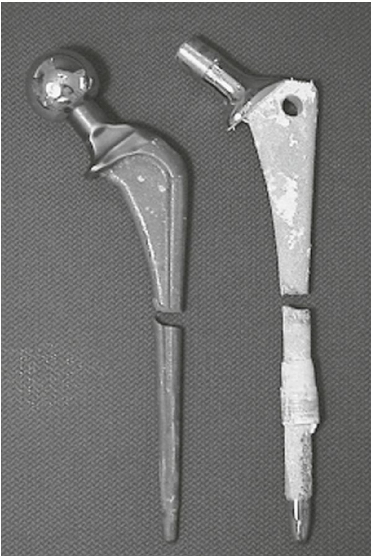
**FIG. 5.18** Photograph of stems retrieved because of stem fracture. Stem on the left was cemented. Stem on the right was cementless. Both stems have narrow diameters, and both fractured in the typical region—the transition to the narrow part of the stem.
