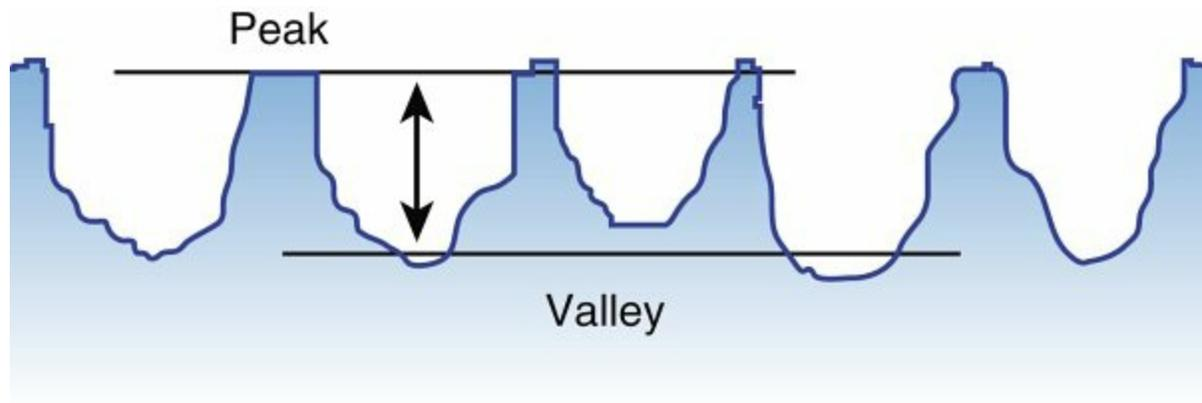
**FIG. 5.13** Surface roughness ( $R_a$ ) of bone ongrowth prosthesis.  $R_a$  is defined as the average peak to valley on the surface of the implant. The value is typically expressed in micrometers ( $\mu\text{m}$ ).
