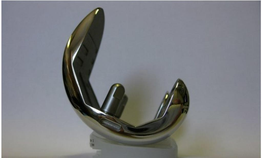
**FIG. 5.79** Lateral view of cruciate-retaining (CR) TKA implant. This is the typical profile of the femoral component. In this design the posterior cruciate ligament is retained. The PE insert is generally more flat to allow the femur to roll back onto the posterior part of the tibial bearing.
