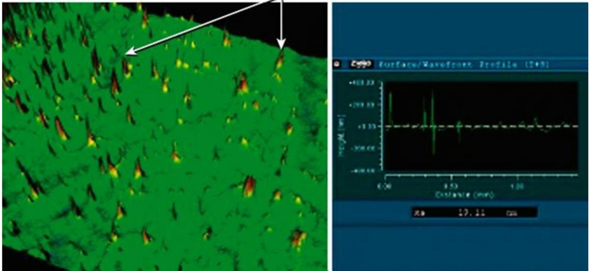
**FIG. 5.37** Scanning photomicrograph of cobalt-chrome (Co-Cr) alloy head. The sharp peaks emanating from the surface are carbide asperities that protrude from the surface. (Courtesy Ian Clarke, PhD, and Donaldson Arthritis Research Foundation.)
